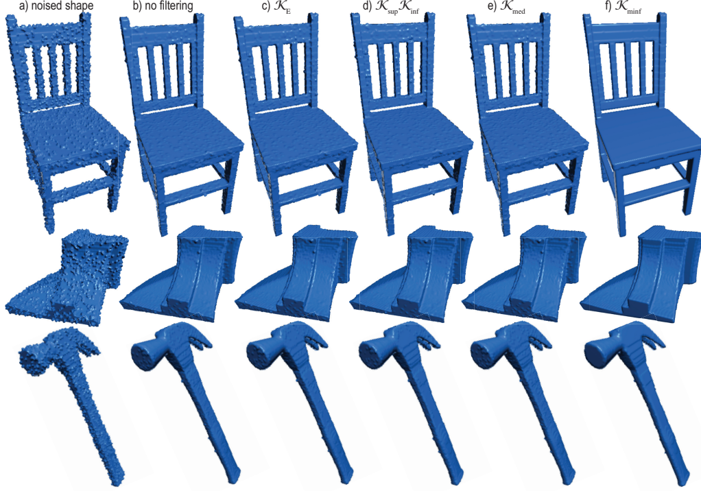
Fig. 9: Comparison of different filters \mathcal{K} for distance transform smoothing. See Sec. 3.3.
